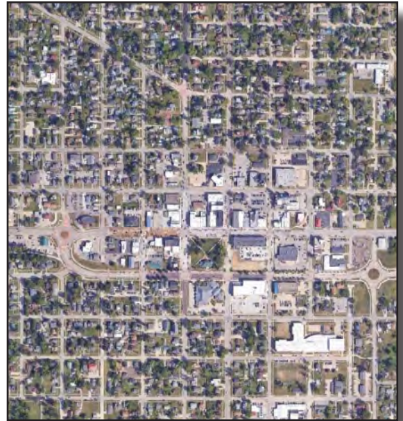
Image 21: Uptown Marion is an example of a traditional street grid. Often, these street networks are uniform and located in the oldest parts of town, as is the case in Marion. Source: Google Maps
