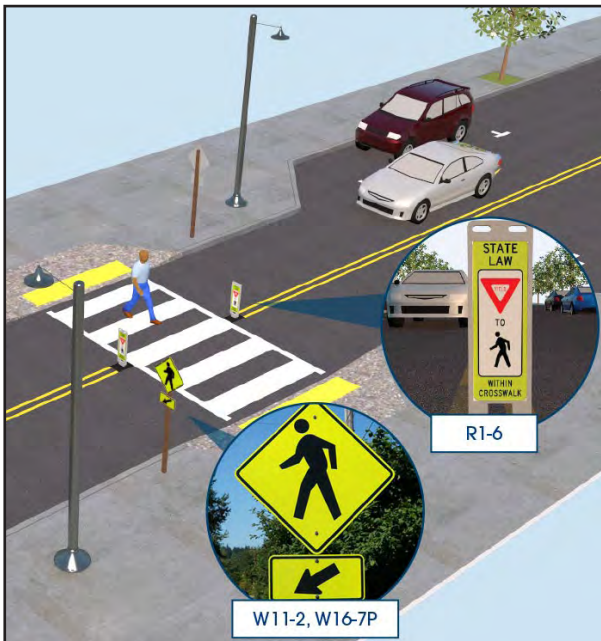
Image 29: Example of a high visibility crosswalk. Source: Federal Highway Administration
