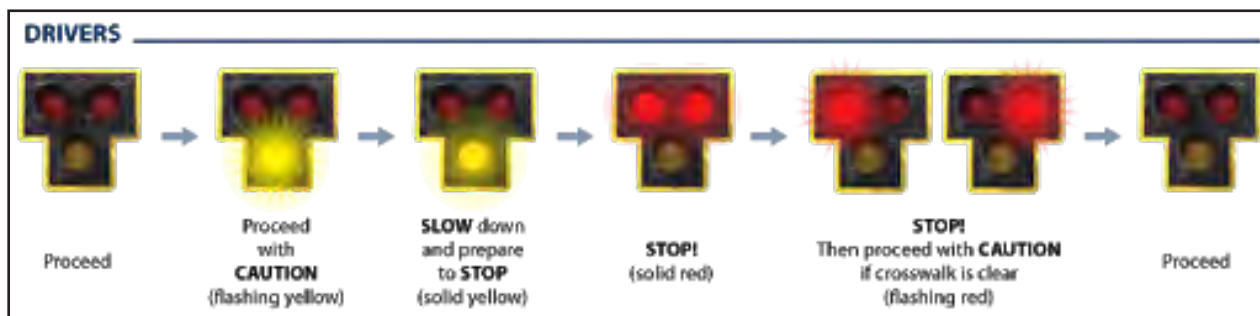
Image 34: Example of a pedestrian hybrid beacon. Source: Federal Highway Administration
